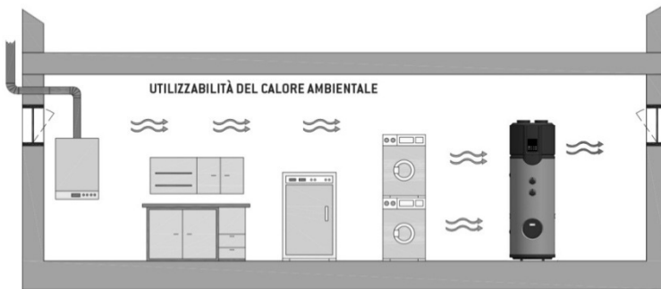
Fig. 7 – Possible solutions when using the heat pump
