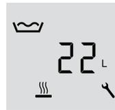
Keep the “Plus” and “Minus” buttons pressed. In addition, press the “Menu” button and keep all three buttons pressed for 5 seconds.
